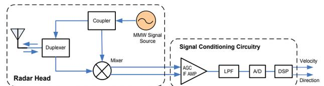
Fig. 2. A typical homodyne Doppler radar set.
