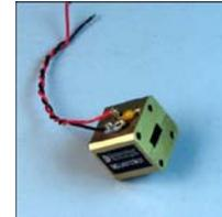
Fig. 4. A photo of sensor front-end module.
