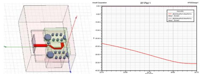
Fig. 6. The dual waveguide-to-microstrip transition model in HFSS and simulated return loss.
