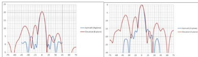
Fig. 7. Antenna gain simulation (left) and measurement results.
