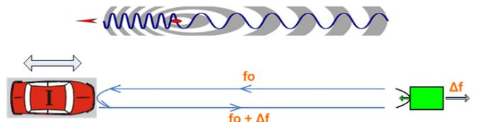
Fig. 1. Speed measurement principle based on Doppler effect.
