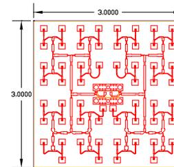
Fig. 5. The designed 24.15 GHz patch antenna.
