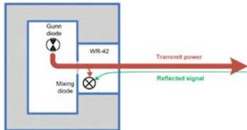
Fig. 3. Sensor front-end module illustration.
