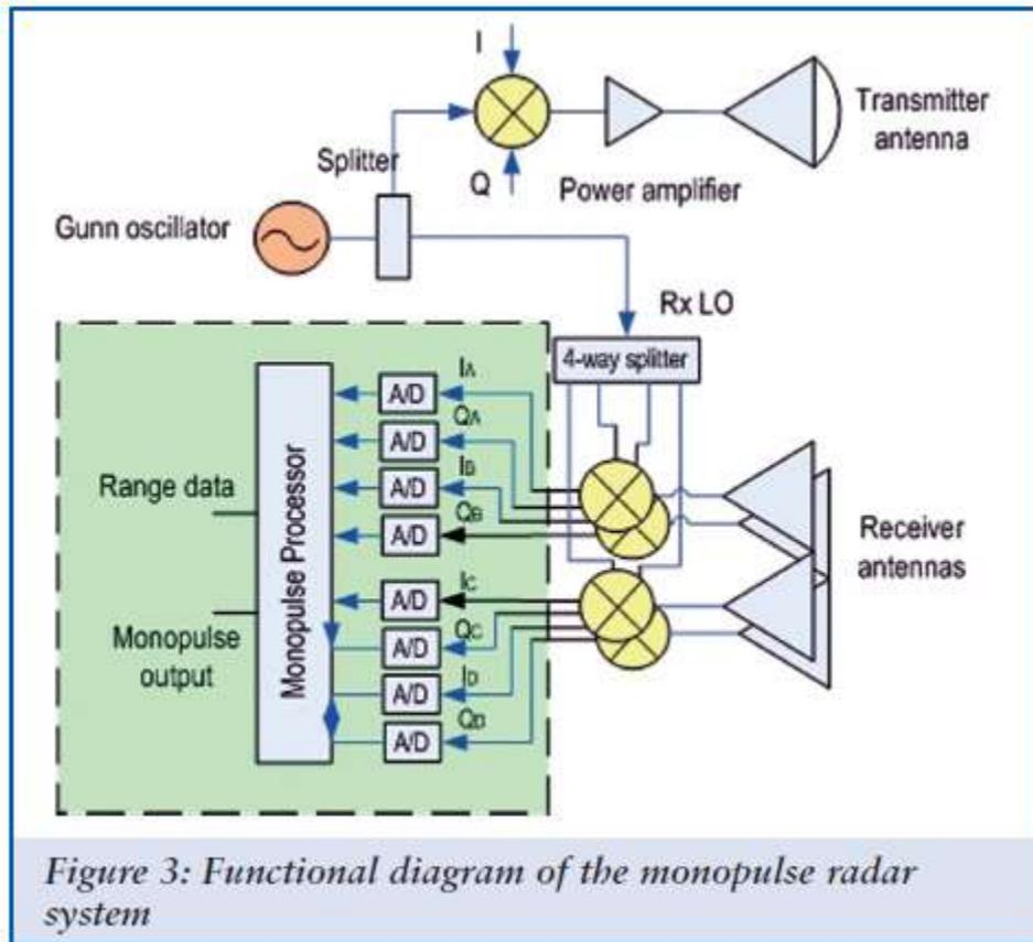
*Figure 3: Functional diagram of the monopulse radar system*
