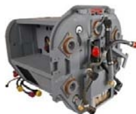
Raytheon AESA Radar Rack
